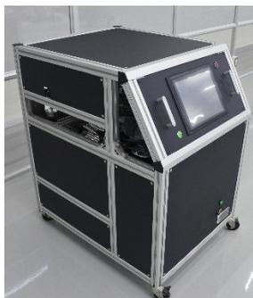
Figure 3: Picture of slow pumping and venting system.
