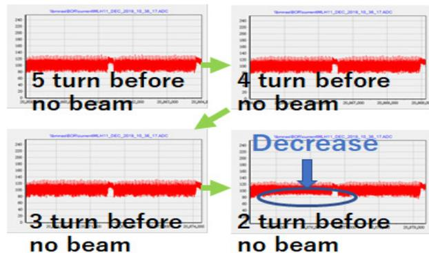
Figure 4: Bunch oscillation monitor signals in a damaged event.
