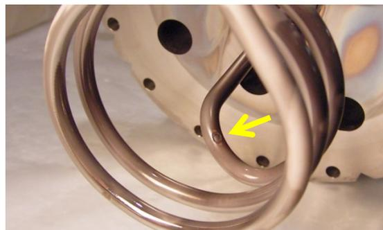
Figure 9: Damage of RF-antenna coating in RUN#82.
