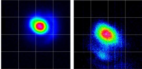
Figure 4: UV laser beam profiles of the 1st and 2nd line at the position of virtual cathode.
