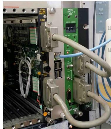
Figure 4: CAMAC controller using optical module.
