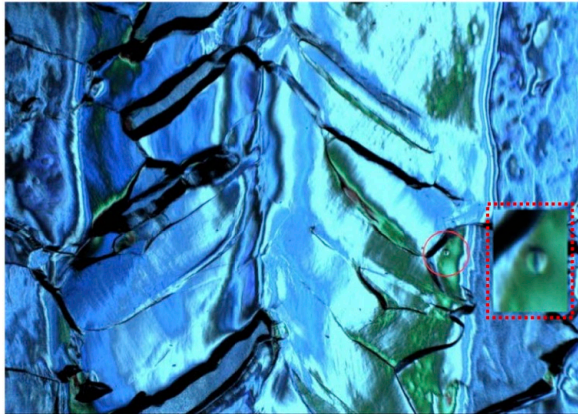
Figure 2: Inner surface photograph of superconducting cavity including defect area taken by inner surface inspection system.
