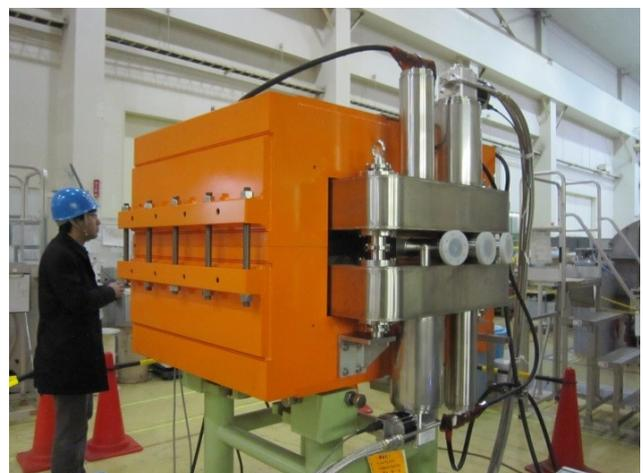
Figure 1: Prototype HTS magnet: HTS-SW1.
