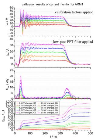
Figure 6: Comparation of the standard waveforms from current transformer and the processed waveforms from current monitor.
