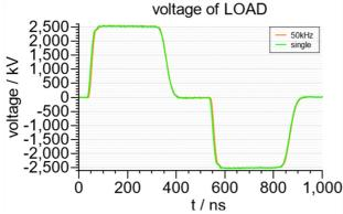
Figure 7: Output voltage of the load at 50 kHz and single shot.
