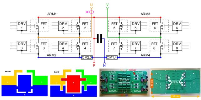
Figure 2: Circuit schematics, structure of buses and picture of the updated design of 4th generation of SPS.
