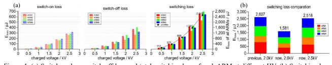
Figure 4: (a) Switch-on loss, switch-off loss and total switching loss of each ARM at different HV. (b) Switching loss comparation of the previous and the updated SPS.
