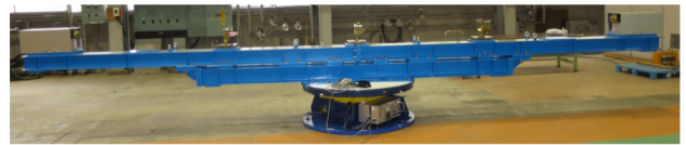
Figure 6: Winding machine for 7 m-long coil.
