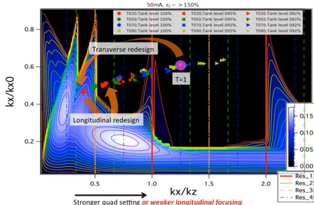
Figure 6: Stability chart for J-PARC ACS section operation tune setting.
