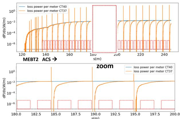
Figure 4: Simulated H0 loss-pattern in MEBT2-ACS.
