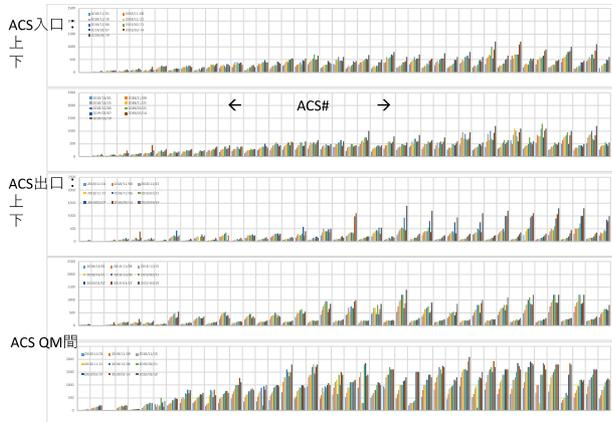
Figure 7a: ACS Residue Radiation on surface at 500kW, linac peak current 50mA in Nov. 2018 to March 2019 at ACS, with baseline design with  $T_x/T_z=1.0$ .
