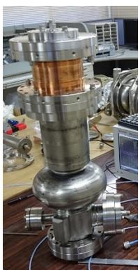
Figure 2: Prototype HOM absorber was connected with the single-cell cavity for RF measurement at room temperature.
