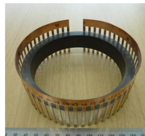
Figure 5: Test piece which brazed an AlN cylinder and thin copper strips. The width of a copper strip is 3 mm.
