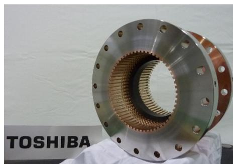
Figure 1: Prototype HOM absorber.
