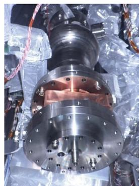
Figure 4: The prototype HOM absorber with the single-cell cavity was installed in the horizontal cryostat.
