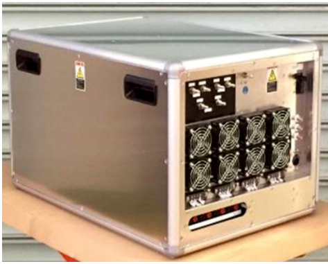
Figure 2: Actual photo of a unit chopper type MARX power supply.
