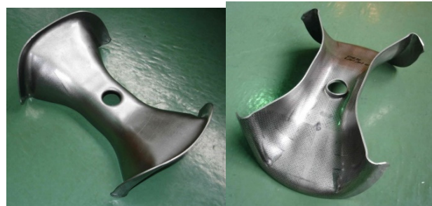
Figure 1: Press formed shape after burring with niobium sheet of 2.5 mm thick.
