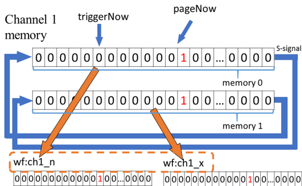
Figure 5: Behavior of double buffer for MR signals.
