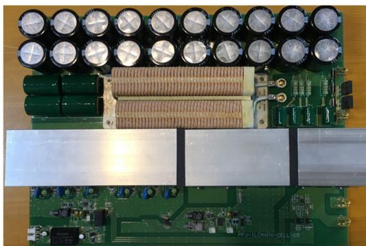
Figure 9: Picture of MARX board after component mounting.
