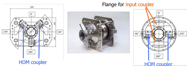
Figure 1: 2cell superconducting cavity using in cERL injector.
