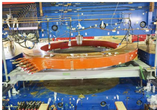
Figure 6: Removing the main coil of the cyclotron.
