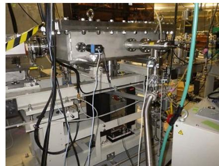
Figure 3: Septum magnet and sputter ion pump.
