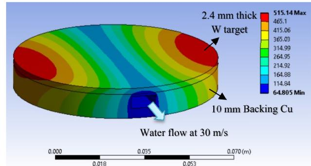
Figure 3: Temperature distribution of the target system.
