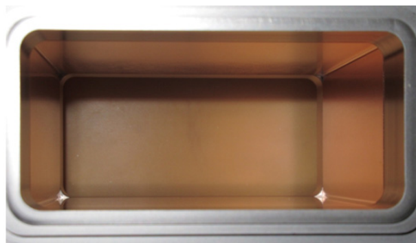
Photo 3: A Photograph of alumina ceramic after high power test by using SLED method.
