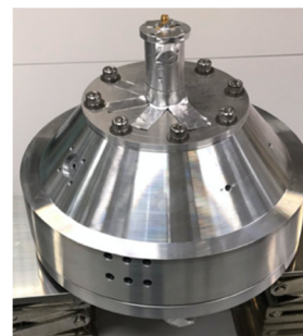
Figure 3 : Mushroom-shaped Aluminum cavity.
