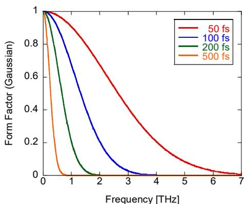
Figure 1: Bunch form factor (Gaussian shape bunch).
