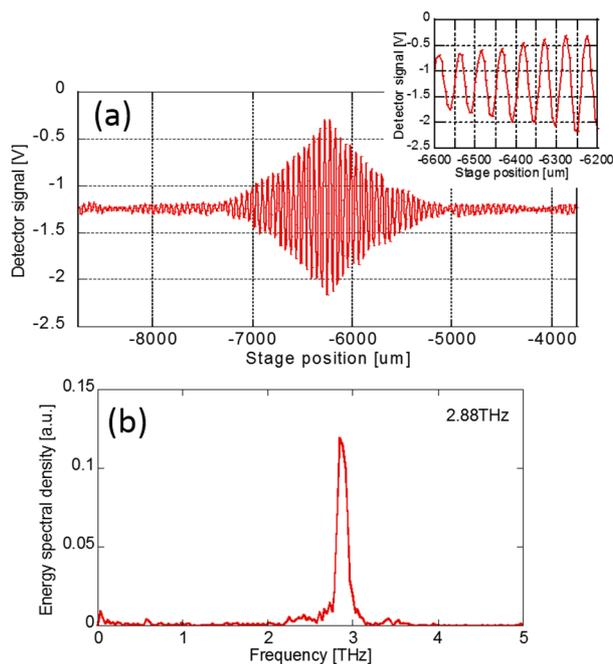
Figure 5: (a) Measured interferogram of undulator radiation. (b) Frequency spectrum of undulator radiation with  $K=3.6$ .
