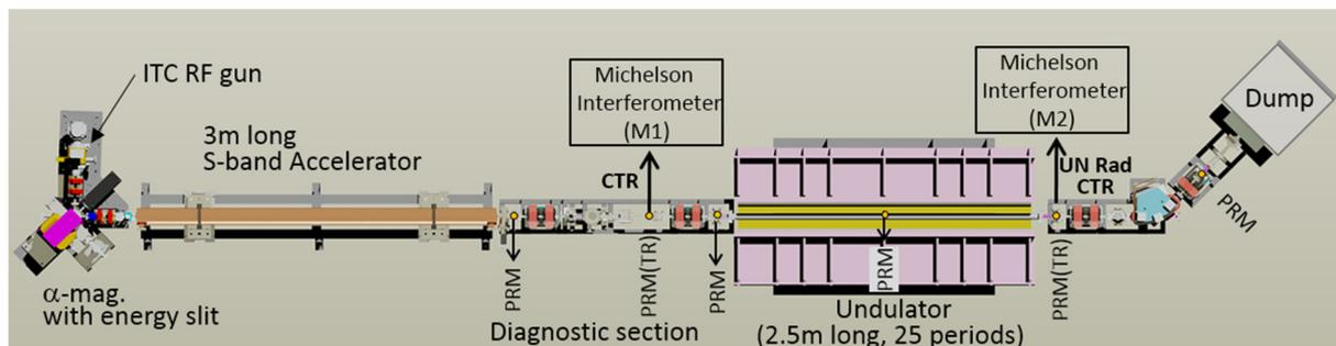
Figure 2: t-ACTS beam line layout.
