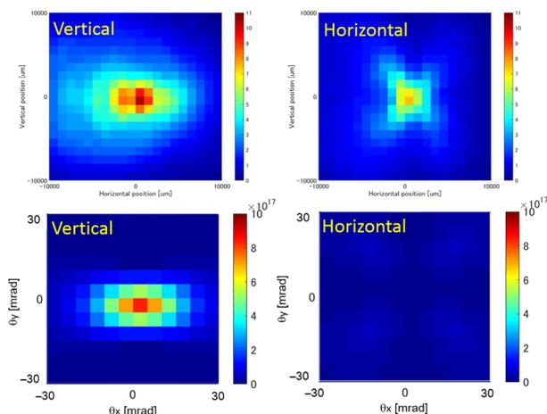
Figure 7: (Upper) Measured spatial profile of undulator radiation using wire grid. Image size is 20mm  $\times$  20mm. Left and right side of profiles are vertical and horizontal polarized component of the radiation, respectively. (Lower) Calculated spatial profiles of undulator radiation from single electron.
