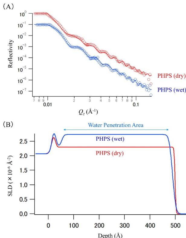
Figure 1: (A) NR profiles of the dry and wet SiO<sub>2</sub>(PHPS) thin layer samples. The circles represent the experimental data, and the solid lines represent the best-fit calculated NR profiles. (B) Depth profiles of the dry and wet SiO<sub>2</sub>(PHPS) thin layer samples calculated by obtained structural parameters.
