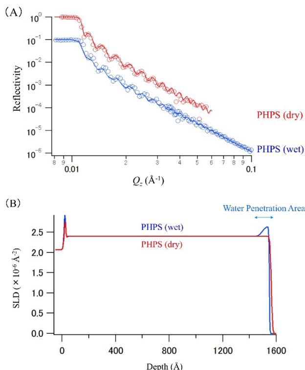
Figure 2: (A) NR profiles of the dry and wet  $\text{SiO}_2(\text{PHPS})$  thick layer samples. The circles represent the experimental data, and the solid lines represent the best-fit calculated NR profiles. (B) Depth profiles of the dry and wet  $\text{SiO}_2(\text{PHPS})$  thick layer samples calculated by obtained structural parameters.
