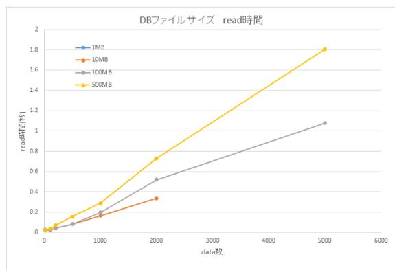
Figure 5: Read performance vs DB file size.
