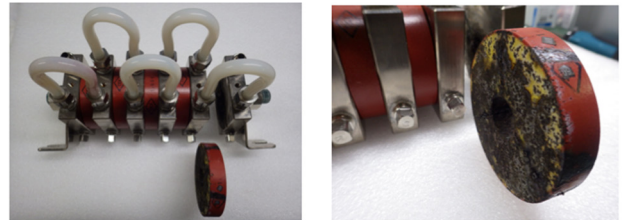
Figure 6: Discharge breakdown of the ceramic resistor unit and its resistor element.
