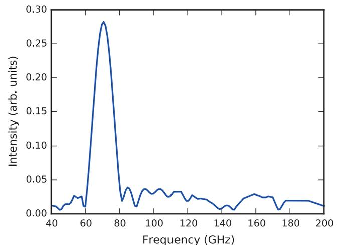
Figure 3: SPR reconstructed spectrum in the range of 60 – 90 GHz.
