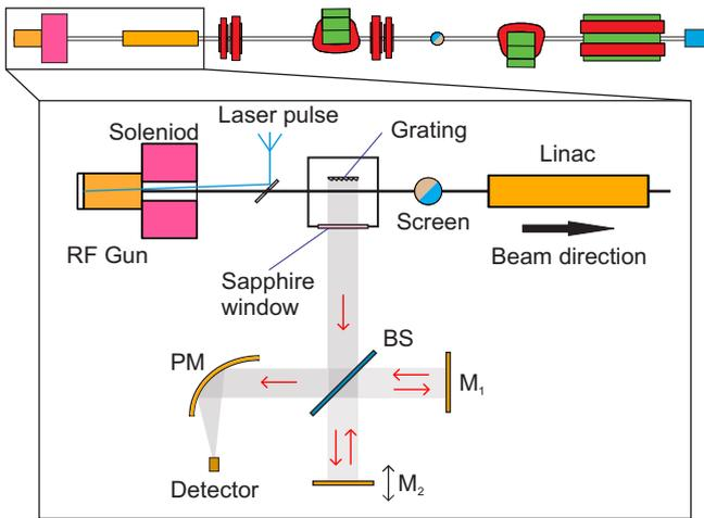
Figure 1: LUCX beamline and experimental schematics. Abbreviations:  $M_1$  - fixed interferometer mirror,  $M_2$  - movable interferometer mirror, BS - splitter, PM - off-axis parabolic mirror.
