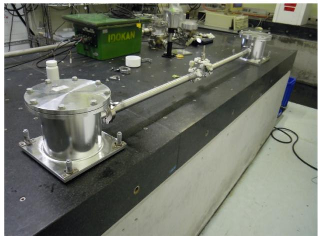
Figure 2: External view of the oil-tube tilt-meter.
