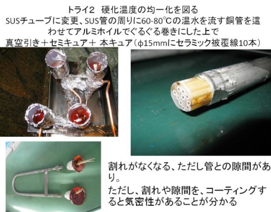
Figure 5: Left: A warm up equipment of SUS pipe by hot water. Right: The sample of 10 signal cables in a φ15 SUS pipe
