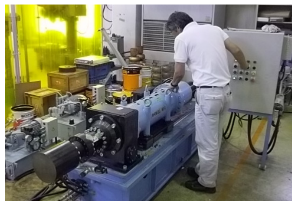
Figure 3: Hydroforming machine (Final hydraulic pressure: 25 MPa).
