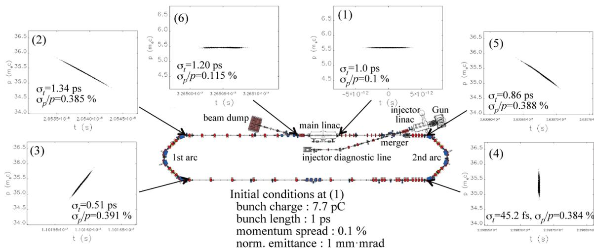
Figure 4: Change of time-momentum ( $t, p$ ) distribution of the electron bunch along the cERL when SX2 and SX4 are used. The numbers on the distribution plots mean their temporal order. The bunch length and momentum spread are also shown on each plot. In the simulation, the bunch length is minimized at the entrance of the 2<sup>nd</sup> arc section (4) and the momentum spread at the entrance of the dump line (6).
