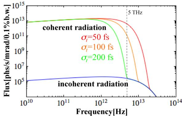
Figure 1: CSR spectra of the 20 MeV cERL for three different bunch lengths of 50, 100 and 200 fs, at the bunch charge of 7.7 pC and the bunch repetition frequency of 130 kHz.
