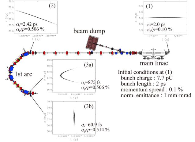
Figure 3: Change of time-momentum ( $t, p$ ) distribution of the electron bunch from before the main linac to after the 1<sup>st</sup> arc section in the bunch compression process. The numbers on the distribution plots mean their temporal order. (3a) and (3b) correspond to two cases of SX1-4 OFF and SX2&4 ON listed in Table 1. The bunch length and momentum spread are also shown on each plot. In the simulation, the bunch length is minimized at the exit of the 1<sup>st</sup> arc section.
