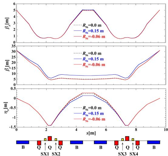
Figure 2: Horizontal and vertical betatron functions ( $\beta_x$ ,  $\beta_y$ ) and dispersion function ( $\eta_x$ ) of the arc sections with three different  $R_{56}$  values of 0.0 m (black broken line), 0.15 m (blue solid line) and -0.06 m (red solid line). B, Q and SX1-4 indicate the bending, quadrupole and sextupole magnets, respectively.
