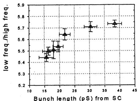
Figure 7. Relation between amplitude of low and high frequency from bottom type BPM.
