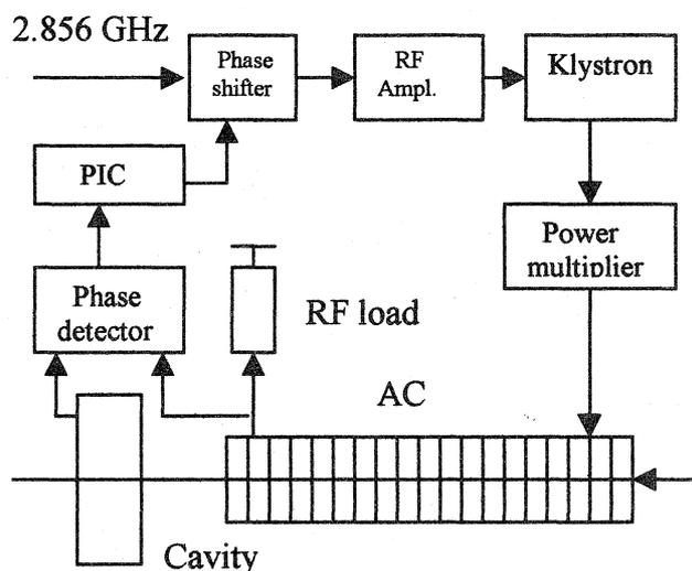
Figure 8. Beam based phase stabilize system
