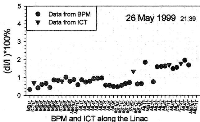
Figure 2. Stability of Intensity along the linac
