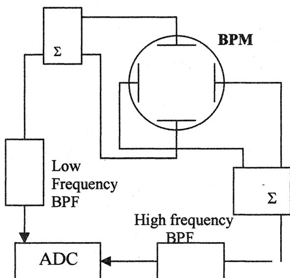
Figure 6. The block diagram of Bunch length measurement.
