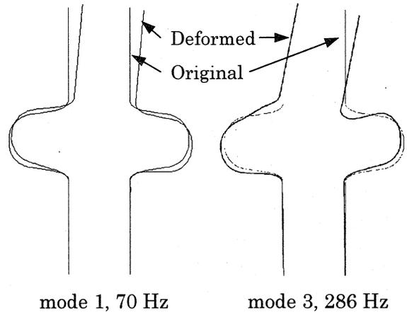
Figure 6 Calculated vibrational modes. (3-dimensional model analysis)
