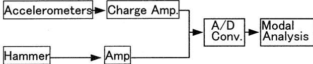
Figure 3 Experimental setup for modal test.
