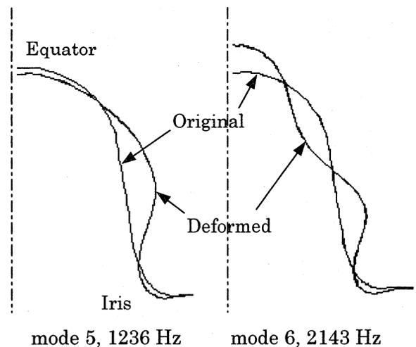
Figure 7 Calculated vibrational modes. (2-dimensional model analysis)
