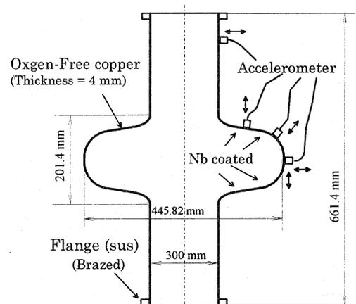
Figure 1 Cavity shape and transducers for vibrational modal test.
