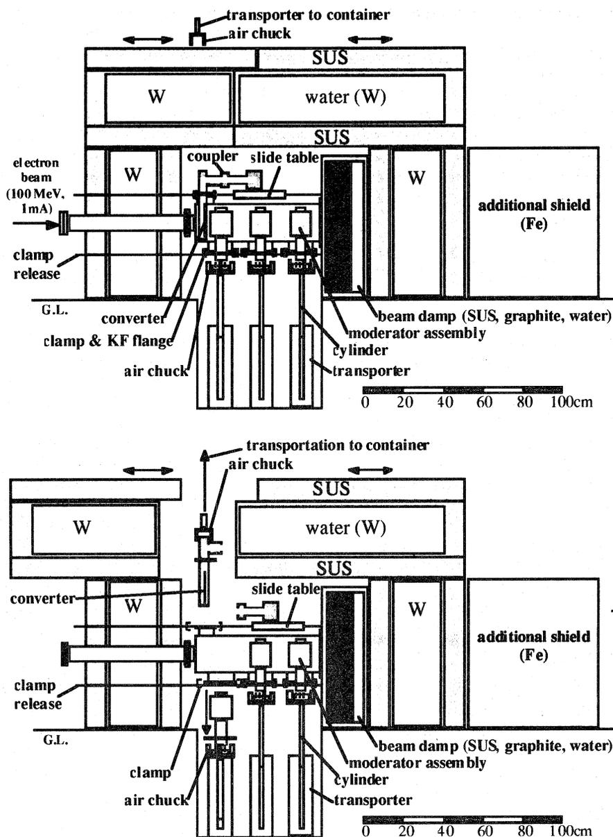
**Fig.2.** A concept of the local shield of the target system and the remote manipulation mechanism.
