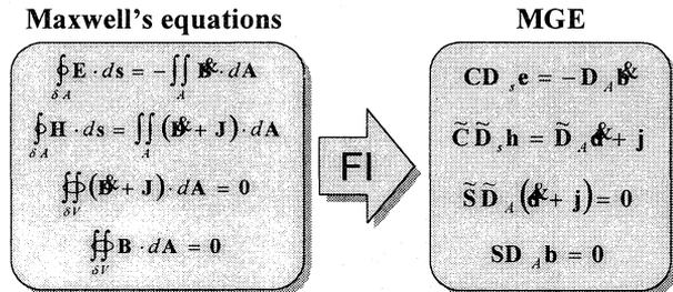
Fig. 1.1: MGE derived from Maxwell's equation by the FI method.
