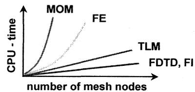
Fig. 1.3: Computation time versus number of mesh nodes for various numerical techniques.
