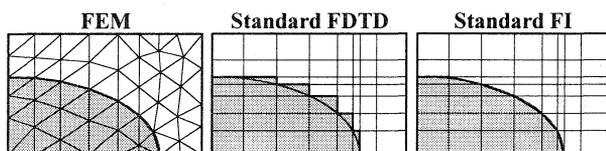
Fig. 1.2: Geometry approximation used in different numerical techniques.
