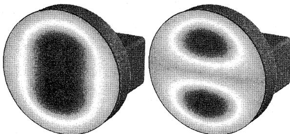
Fig. 3.1.2:  $|E|$  of  $TE_{11}$  (left) and  $TM_{11}$  (right) like modes on the surface of the ceramic disc in the SLAC Type RF Window.
