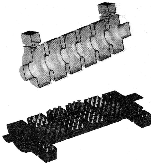
Fig. 3.2.1: Mesh model of a 6-cell Traveling Wave Accelerator (above) and magnetic field of the  $\pi$  mode in a cross section (below).
