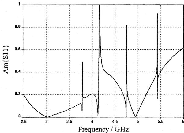
Fig. 3.1.1: Amplitude of S11-parameters of the SLAC Type RF Window.
