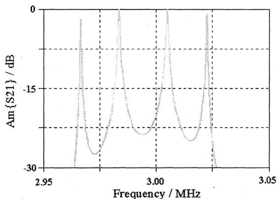
Fig. 3.2.2: Amplitude of S21 of the 6-cell Traveling Wave Accelerator.
