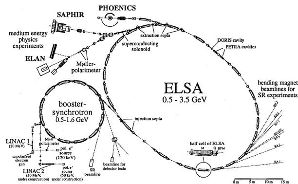
Fig. 1: Site plan of the ELSA facility at Bonn University
