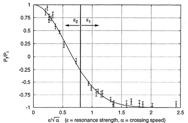
Fig. 2: Ratio of the polarization before and after crossing of the third imperfection resonance versus  $\epsilon/\sqrt{\alpha}$ .
