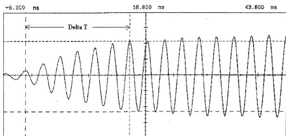
Fig.4 Measured rise time ( $\Delta T$ ) of the RFD cavity.
