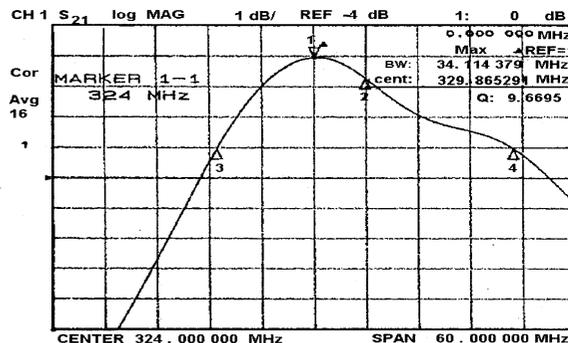
Fig.5 Spectrum of  $S_{21}$  showing the  $Q_L=9.7$
