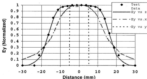
Fig. 3  $E_y$  field distribution in three directions ( test data is in z direction).
