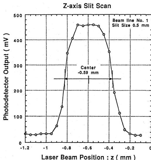
Fig. 2. Z-axis slit scan. The slit center is found at  $-0.59 \text{ mm}$ . We move the z-axis of the mirror No. 1 to this center.
