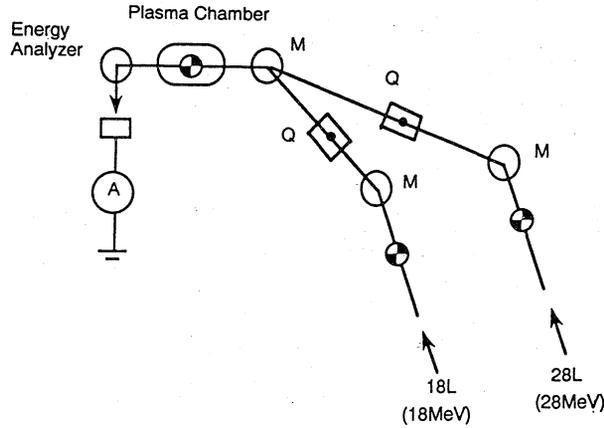
Fig. 2 Experimental setup of plasma section.
