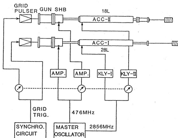
Fig. 1 Schematic diagram of twin linac system at university of Tokyo.
