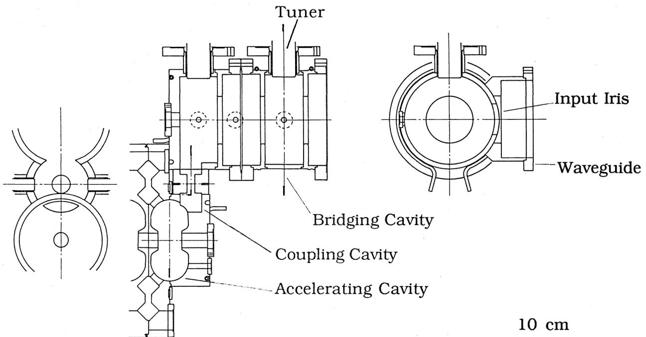
FIGURE RF Structure of Bridge Coupler
