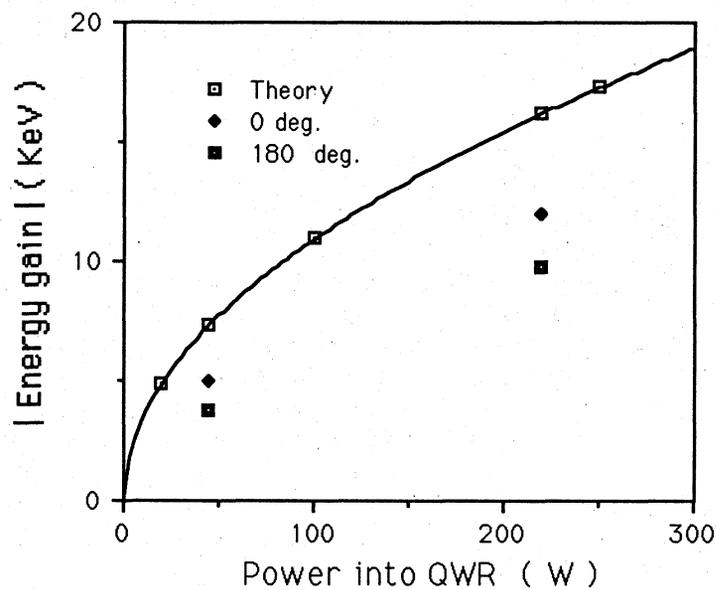
Fig.5: Plot of the absolute energy gain as a function of the input power to the QWR. The theoretical curve is determined from the shunt impedance, 1.2 M ohm.
