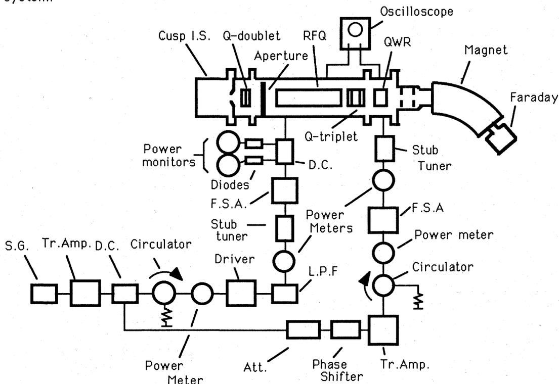
Fig.3 : Schematic representation of QWR test-stand.
