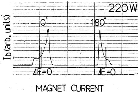
Fig.4: A typical momentum spectrum of the output beam of the QWR . 220 w RF power is delivered into QWR in both "in-phase" ( 0 deg.) and "out-of-phase" ( 180 deg.) situations.
