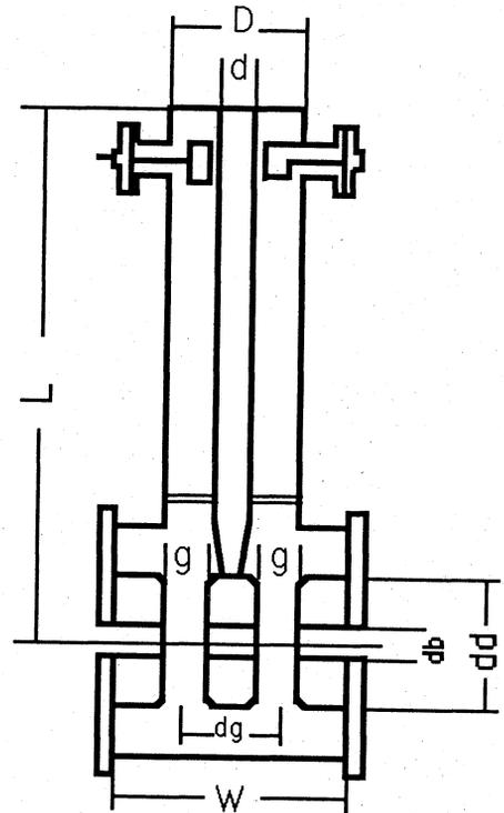
Fig.2: Schematic drawing of the QWR.
