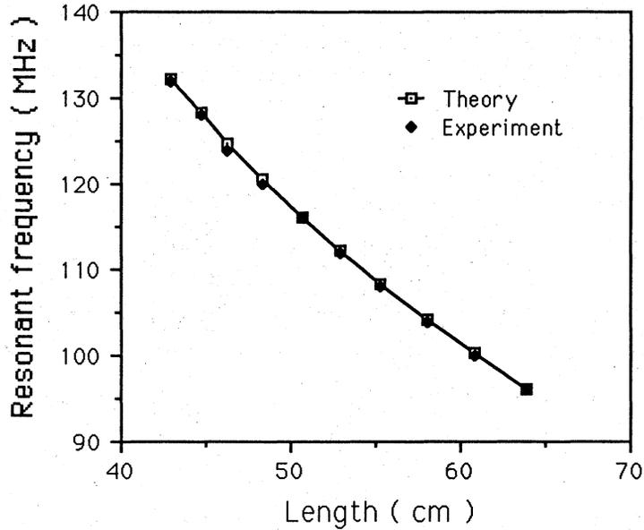
Fig.1: A plot of the resonant frequencies as a function of the coaxial length of the QWR. This is the results of a cold model.
