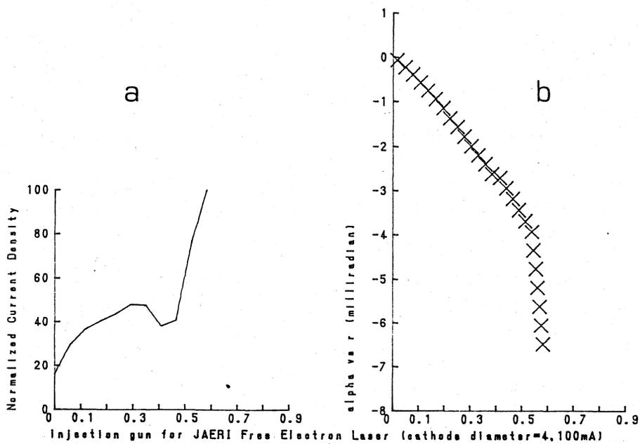
Fig. 2. a) Normalized current density as a function of radial point.
