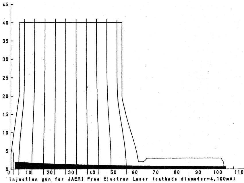
Fig. 1. Shape of the problem region boundary and the equi-potential lines for the cathode with 4mm diam and 100 mA peak current. The filled area near axis shows the beam trajectories from the virtual cathode. Unit is shown in mm.
