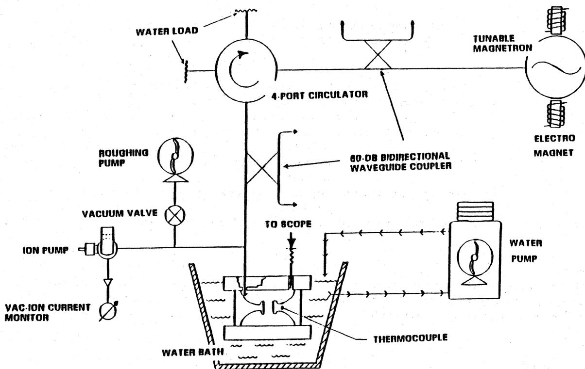
Fig. 3 A schematic diagram of the high power test set-up.
