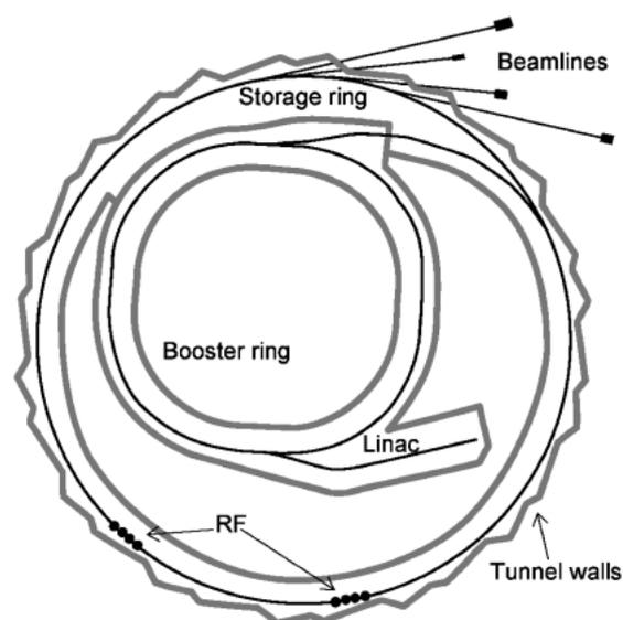
**Fig. 3** The storage ring and injector floor plan
