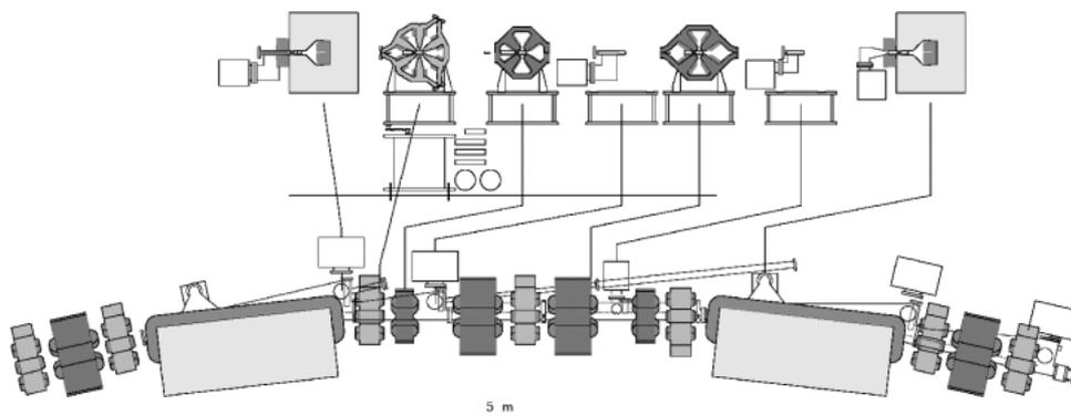
**Fig. 1** A unit cell of the 14 cell double bend achromat ASP storage ring lattice.
