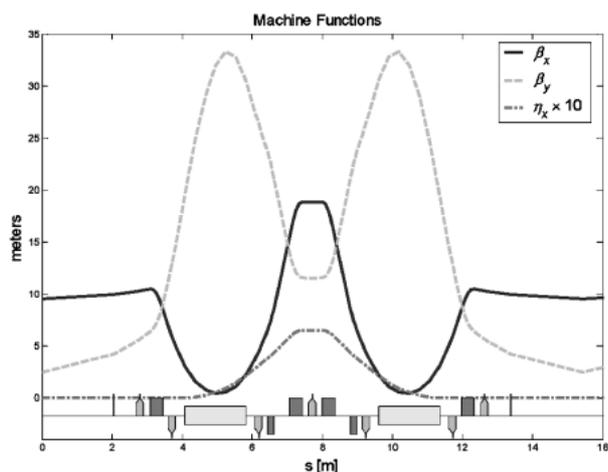
**Fig. 2** Machine functions for one cell of the ASP storage ring with zero dispersion in the straight sections.
