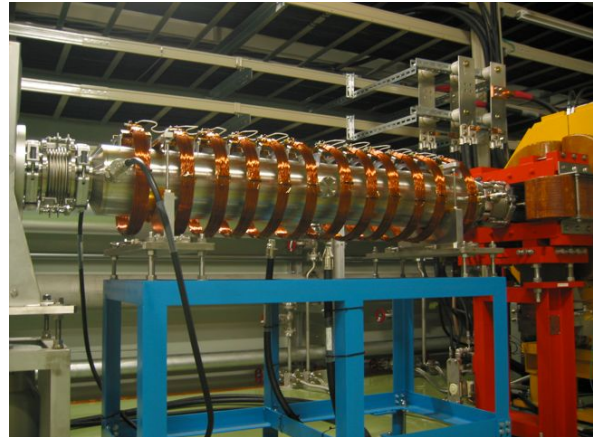
Figure 10: Setup of solenoid around the MR exciter.
