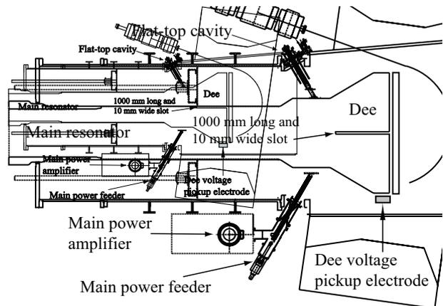
Figure 2: Cross-sectional view of the accelerating system of the RCNP AVF cyclotron.
