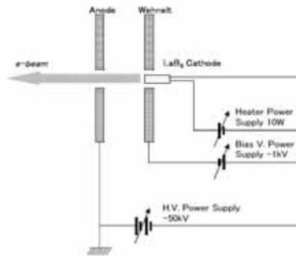
Figure 1: The schematic diagram of DC gun system.
