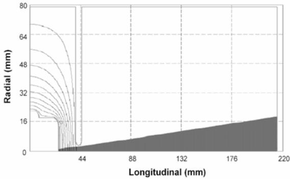
Figure 6: Extraction of an electron beam of 300 mA in a DC electron gun according to a simulation with EGUN.
