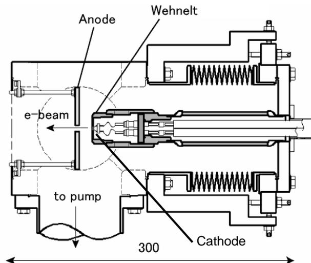
Figure 2: The low emittance DC electron gun.
