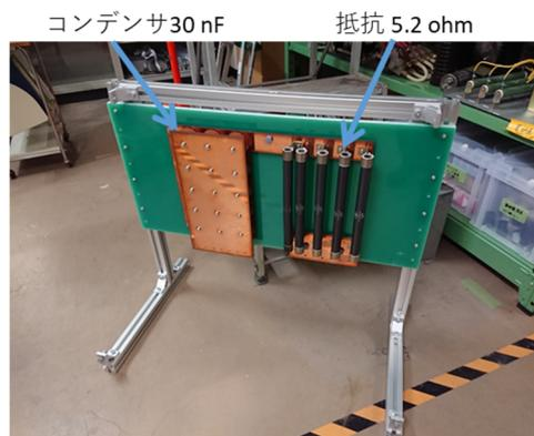
Figure 7: RC circuit.
