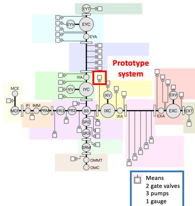
Figure 5: Figure of vacuum system for KAGRA.
