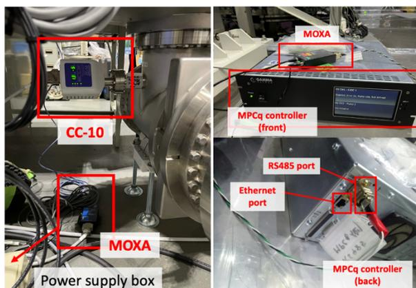
Figure 2: Real implementation of a CC-10 controller, a MOXA server (left), and an ion pump controller (MPCq controller) (right).
