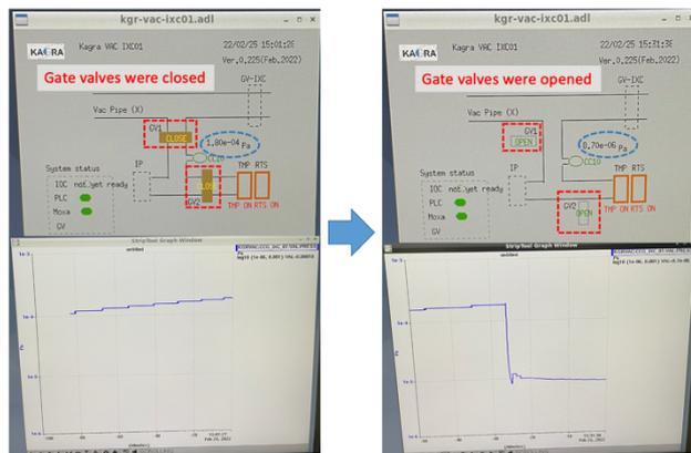
Figure 4: The upper picture shows the GUI of the prototype system. The lower picture shows the pressure change caused by the opening gate valves. The trend graph is by an EPICS tool, StripTool.
