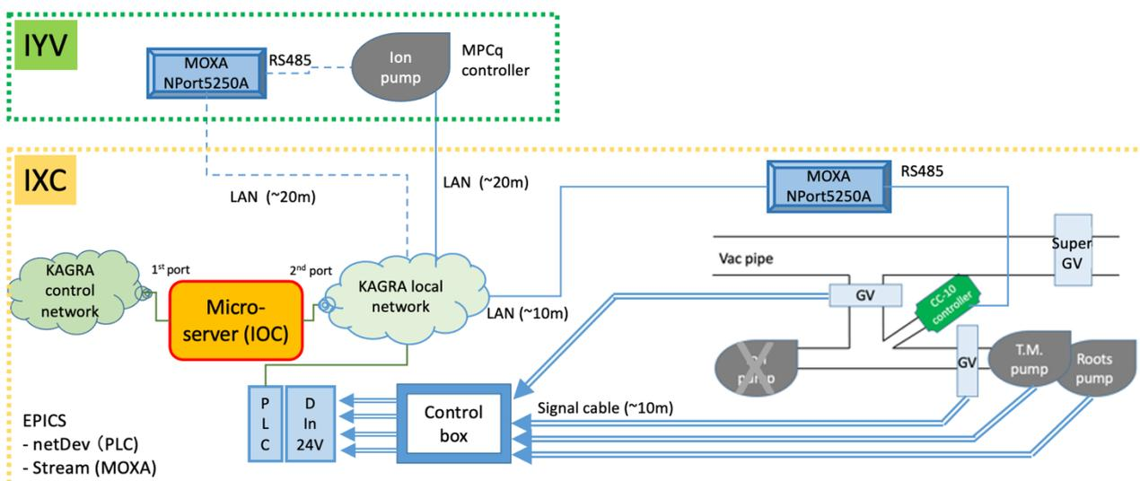
Figure 1: The structure of prototype monitoring system of KAGRA.
