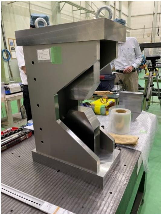
Figure 9: Photograph of test dipole electromagnet.
