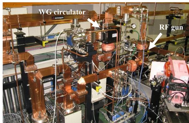
Figure 3: WG system for ITC-RF gun in injector linac.
