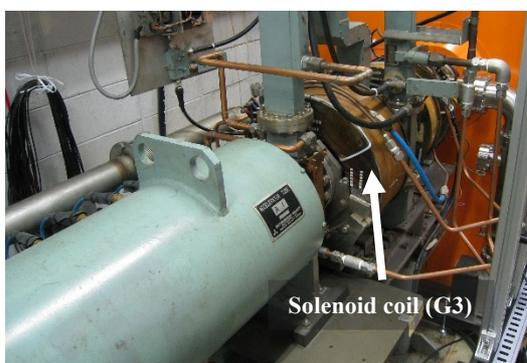
Figure 2: Solenoid coil (G3) in high intensity linac.
